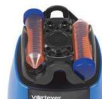
25 mL, 50 mL conical tubes x 2 (horizontally mounted)
